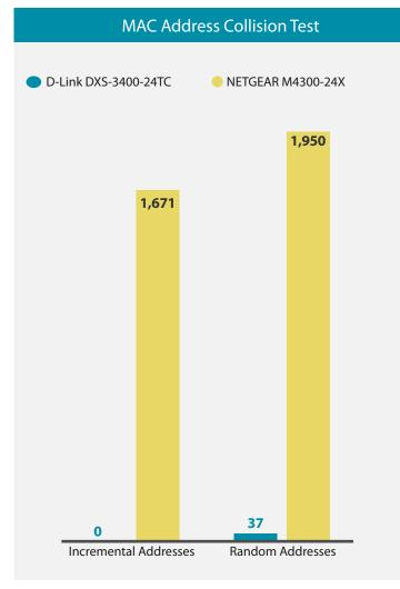
Note: D-Link specifies support for 48K MAC addresses, 32,768 were sent in each test. NEATGEAR specifies support for 16K MAC addresses, 16,000 were sent in each test. (As reported by IxiaNetwork v8.20)
