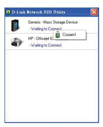
The D-Link Network USB Utility displays which user is virtually connecting this USB device.
