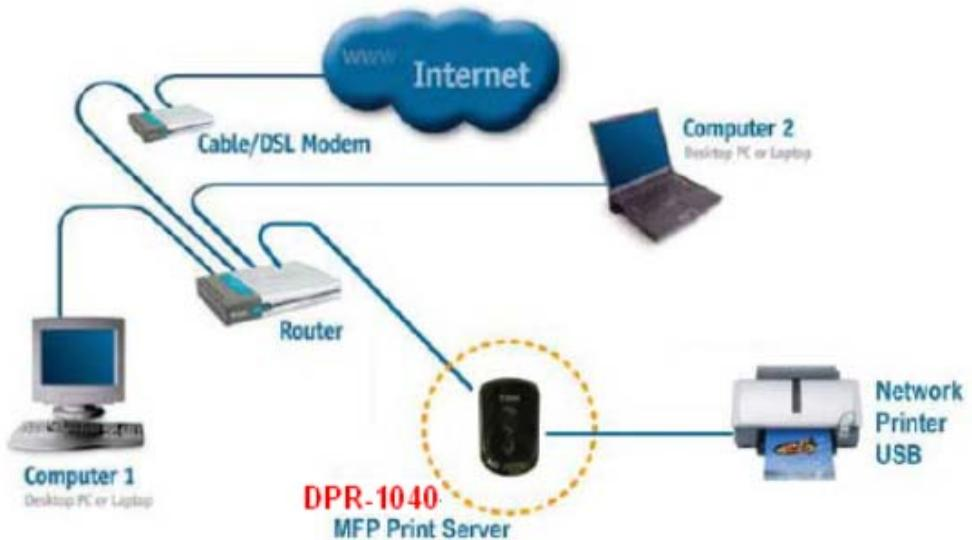
**WARNING:** Only a USB printer may be connected to the USB port of the DPR-1040. Do not connect any other USB devices to the USB port of the DPR-1040; to do so, may damage the unit and will void the warranty for this product.
