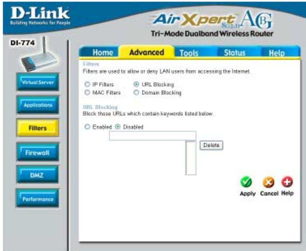
URL Blocking is used to deny LAN computers from accessing specific web sites. A URL is a specially formatted text string that defines a location on the Internet. If any part of the URL contains the blocked word, the site will not be accessible and the web page will not display.
