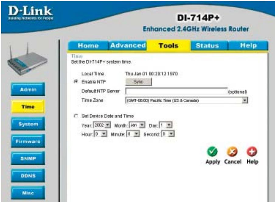
You will need to set the time zone corresponding to your location. The time can be set manually or the device can connect to a NTP (Network Time Protocol) server to retrieve the time.
