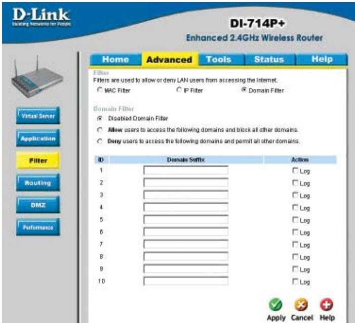
Use Domain filters to allow or deny computers access to specific Internet domains whether it is through www, ftp, snmp, etc. Domain filters apply both to wired computers connected to one of the four Ethernet LAN ports and also to wireless clients connected wirelessly to the DI-714P+.
