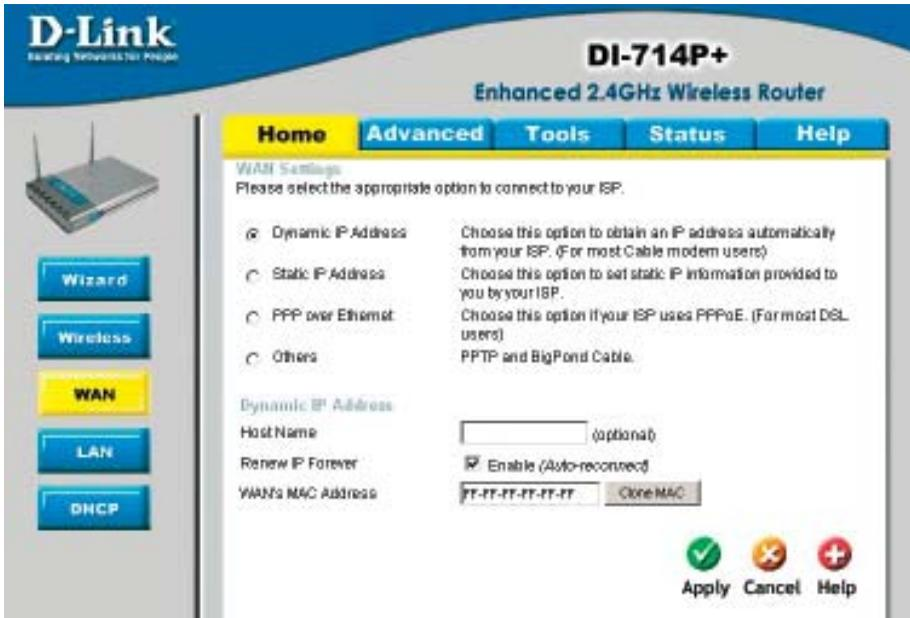
Most Cable modem users will select this option to obtain an IP Address automatically from their ISP (Internet Service Provider).
