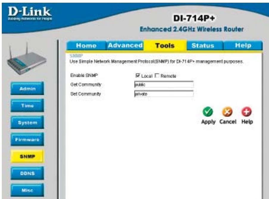
SNMP (Simple Network Management Protocol) is a widely used network monitoring and control protocol that reports activity on each network device to the administrator of the network. SNMP can be used to monitor traffic and statistics of the DI-714P+. The DI-714P+ supports SNMP v1.
