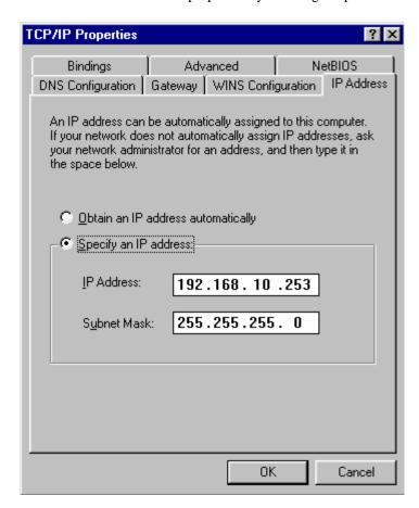
Select specify an IP address and Subnet mask (IP address should be a valid IP address for your network and the Subnet mask should also be the right one for the IP address).
