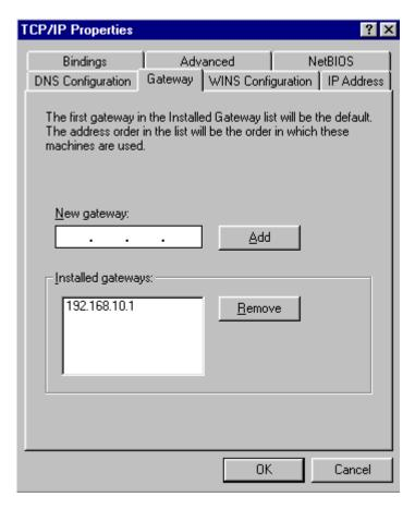
The gateway will be the IP address of the router. So make a note of the gateway that you enter as you will need it later on.
