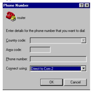
Set connect using to direct to the com port that you are using. (I have got the router connected to com port 2) then do OK.
