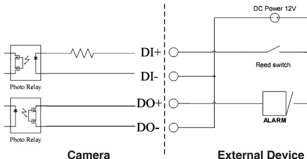
As the Digital Input signal is controlled by an external device, we recommend that you set your device to feed no current normally, and feed a 12V current only to trigger a DI event on the DCS-5605/5635.
