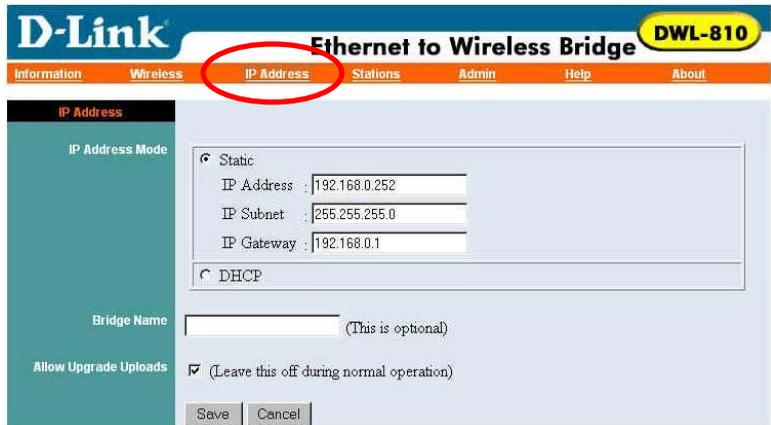
The screenshot shows the D-Link DWL-810 web configuration interface. The top navigation bar includes 'Information', 'Wireless', 'IP Address' (circled in red), 'Stations', 'Admin', 'Help', and 'About'. The main content area is titled 'IP Address' and contains the following settings:
