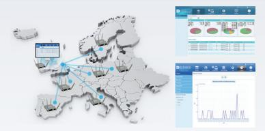
Manage up to 500 APs from a single location, complete with a multitenant structure that provides multi-layer management authority. Allows you to be in control of your wireless network from anywhere in the world through the Internet by using a web browser on your PC, smartphone or tablet. Enterprise-level features such as bandwidth optimisation, captive portal and RF optimisation help satisfy the needs of the modern business environment.
