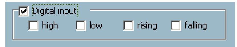
**High:** Checking this will trigger recording while the digital input is high. The technical name for this event is line trigger.
