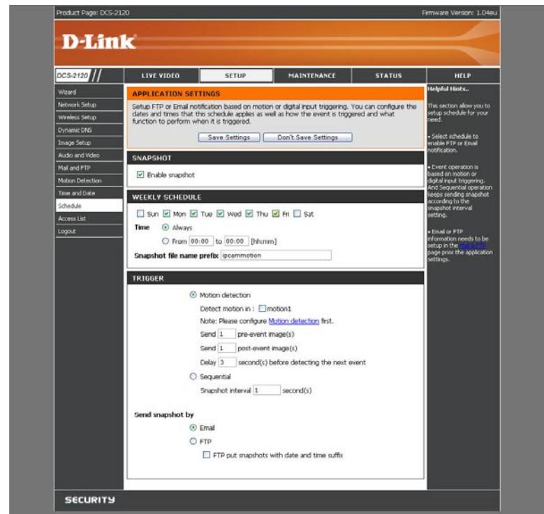
**Detect Motion in:** Check the motion detection window(s) to enable motion triggering. The window(s) can be created in the **Advanced > Motion Detection** page.
