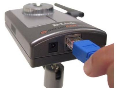
Attach the external power supply to the DC power input connector located on the Network camera's bottom panel (labeled 5VDC) and connect it to your wall outlet. When you have a proper connection, the LED will light up.
