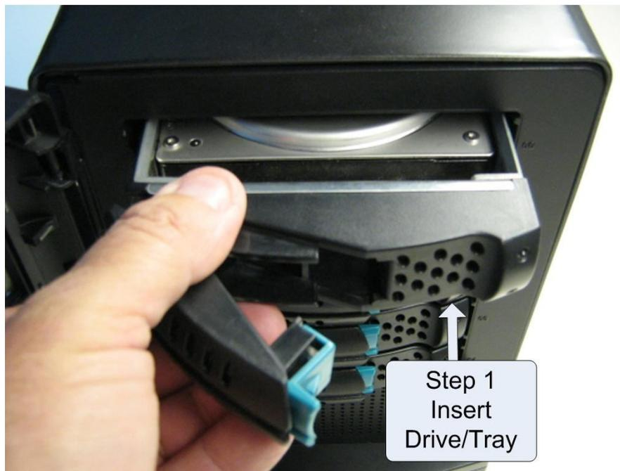
Figure A-21 Drive/Tray Installation
