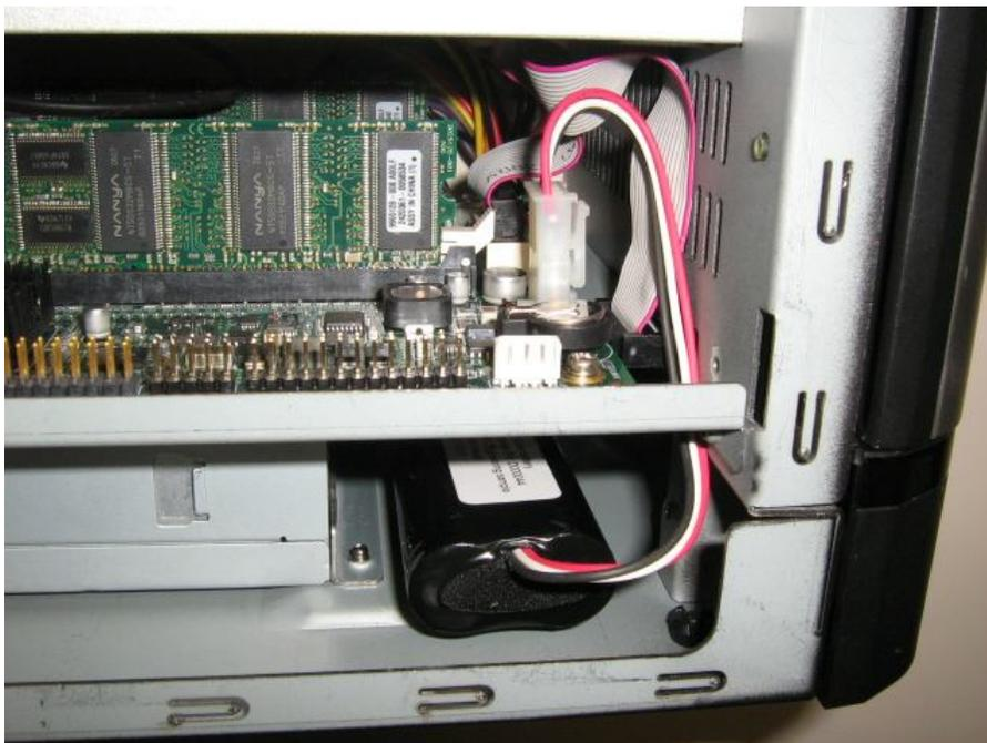
**Figure A-9 The Installed Battery**
