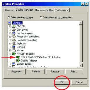
To check that the installation of the DWL-520 was successful, scroll down in the "Device Manager" window and click on "Network Adapters." You have a successful installation when "D-Link DWL-520 Wireless PCI Adapter" appears as shown above.
