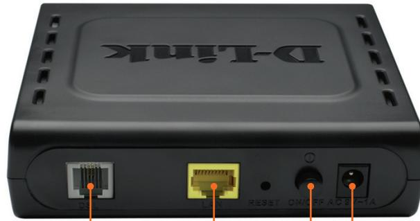
RJ-11 ADSL Port RJ-45 Ethernet Port Power ON/OFF Switch Socket for Power Adapter
