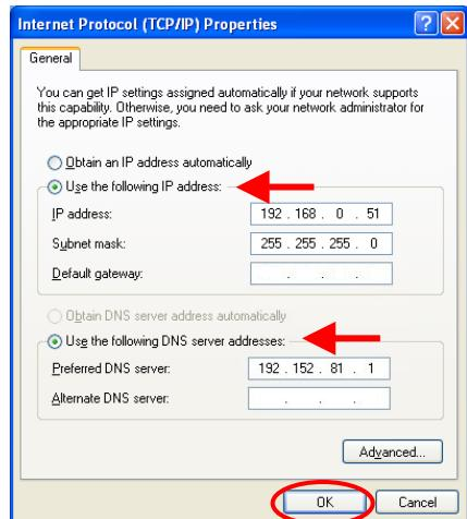
Select **Use the following DNS server address**. Enter the LAN IP address of the Wireless Router.
