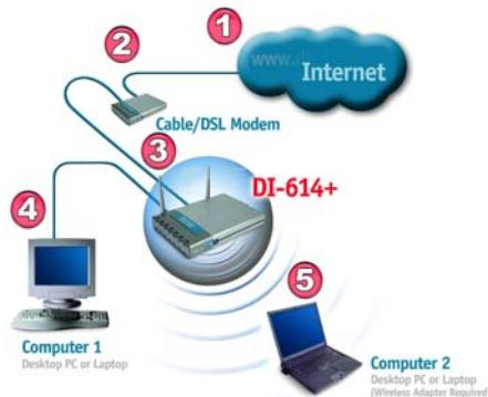
Please remember that **D-Link AirPlus** wireless devices are pre-configured to connect together, right out of the box, with the default settings.
