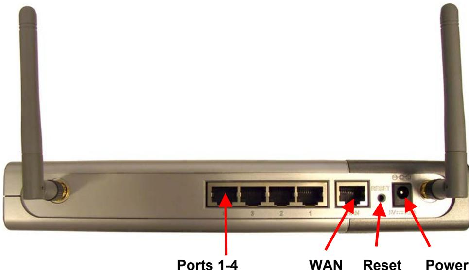
**Reset:** Used to restore the DI-614+ to the factory default settings
