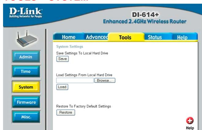
local hard drive and locate the system file to be used. You may also reset the Broadband Router back to factory settings by clicking on **Restore**.
