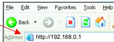
(The IP Address shown in the example above is the default setting. If you have changed the IP Address of the DI-614+ to conform to a network, then input that IP Address in the web browser, instead of the default IP Address shown.)
