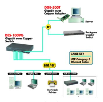
Above is a sample configuration utilizing the power of the DGE-500T Gigabit over Copper Adapter
