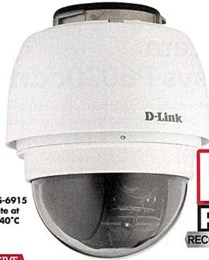
• The DCS-6915 can operate at down to -40°C
