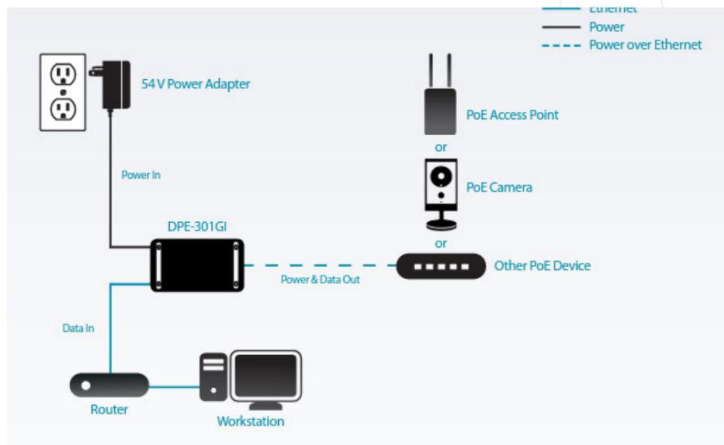
1. Up to 500 m extension requires 802.11at PSE source. Maximum distance as per IEEE 802.3u specifications. Distances exceeding 100 m can be reached by linking additional DPE-302GE units.
