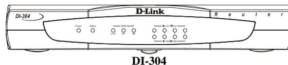
**POWER**— Comes on as soon as you connect the router to the power adapter and plug the power adapter into a suitable AC outlet.
