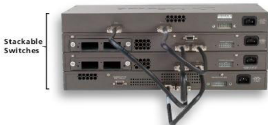
xStack™ - Ring (Bus) Architecture
