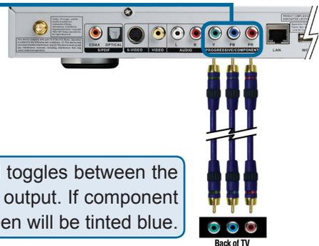
The **VIDEO OUT** button on the remote control toggles between the composite/S-Video output and the component output. If component connectors are used but not selected, the screen will be tinted blue.
