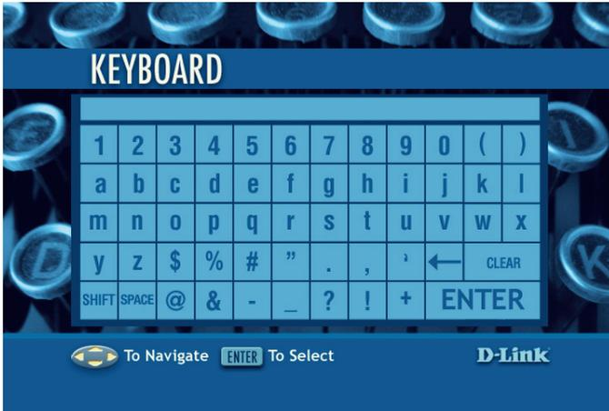
The keyboard is used for a variety of functions such as naming your DSM-320RD and performing searches for music, photos or video. To use the keyboard, highlight a character with the **arrow** buttons on the remote control and press the **ENTER** button. Text can also be entered by using numbers 2-9 on the remote, just as you would on a cell phone. Highlight **ENTER** and press **ENTER** when you're finished entering text.
