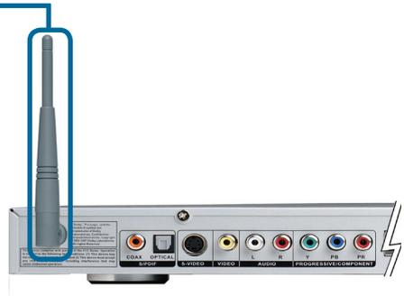
Note: You may have an Ethernet cable plugged into the unit and have the wireless antenna connected. Neither will interfere with the other, but only one network can be accessed at a time (wired or wireless). The network connection type is selected in the Setup Wizard and can be changed by going to the Setup Menu. To access the Setup Menu, press the SETUP button on the remote control.
