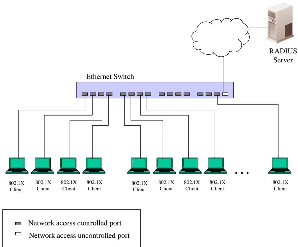
**Figure 7- 21. Example of Typical Port-Based Configuration**
