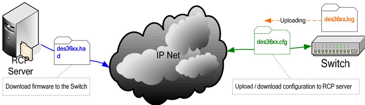
**Figure 2- 39. Remote Copy Protocol between an RCP server and an Ethernet Switch**
