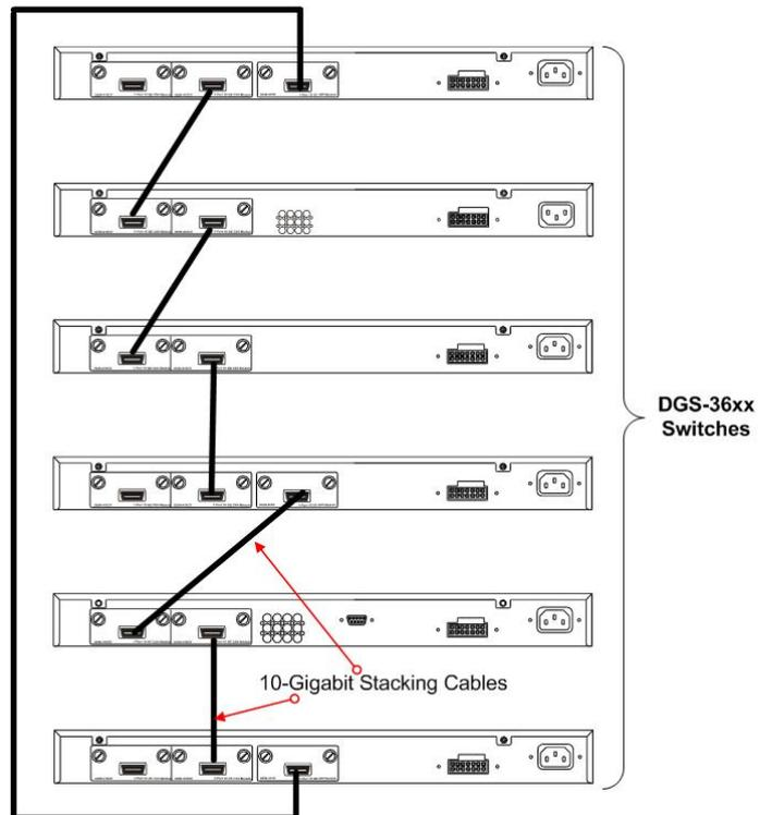
Figure 2- 5. Switches stacked in a Duplex Ring
