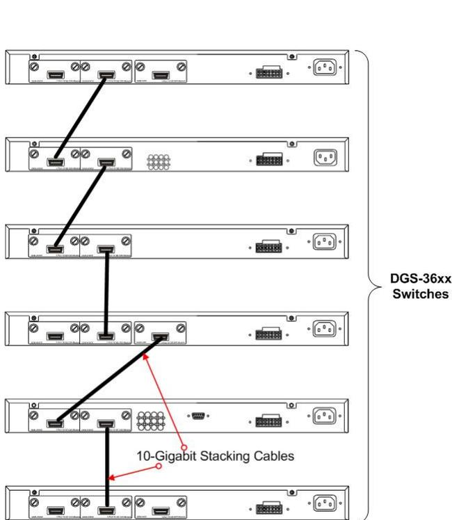
Figure 2- 4. Switches stacked in a Duplex Chain
