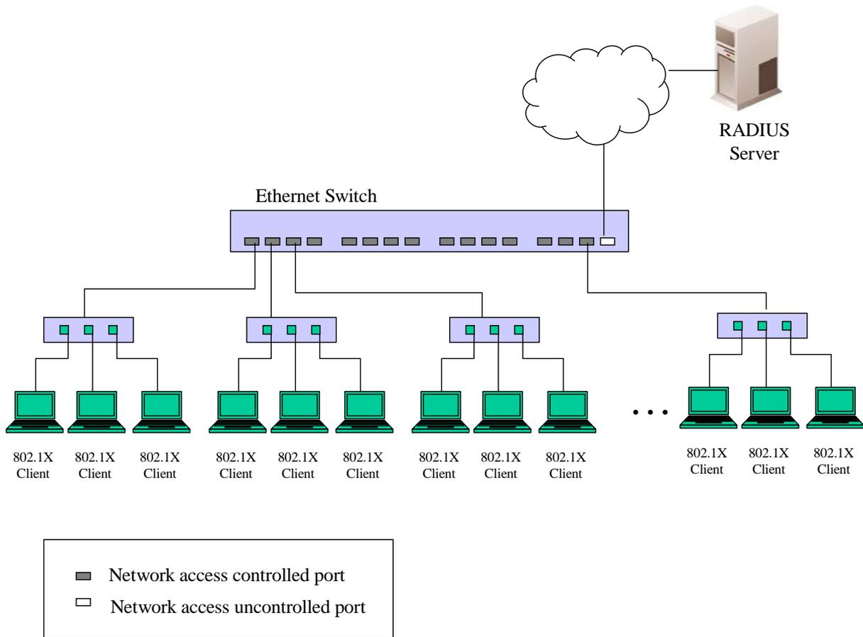
**Figure 7- 22. Example of Typical MAC-Based Configuration**
