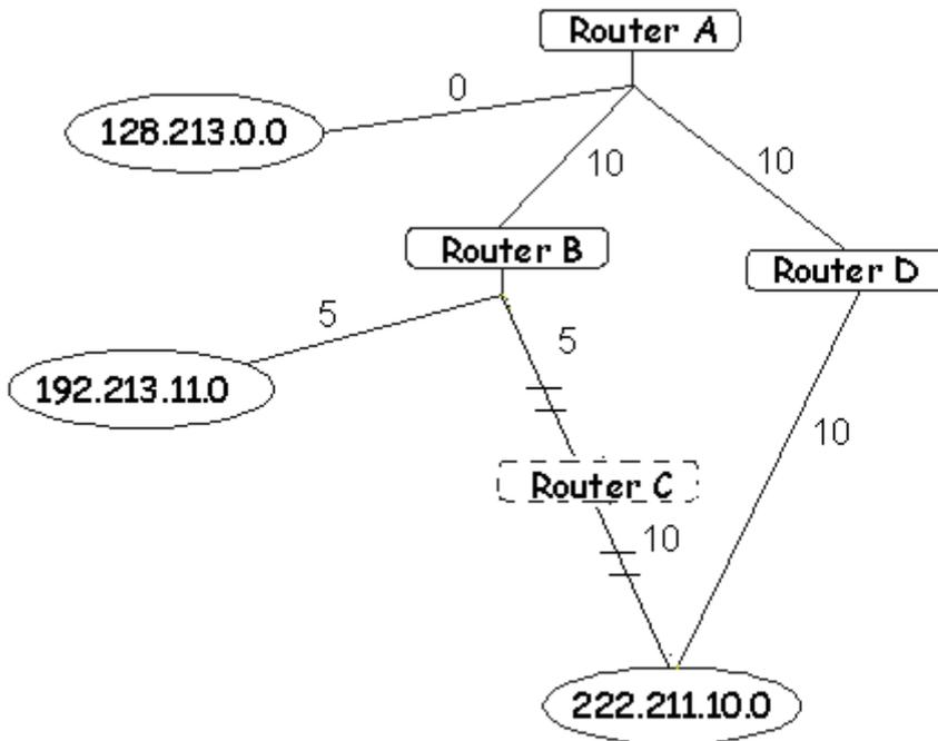
Figure 4- 37. Constructing a Shortest Path Tree
