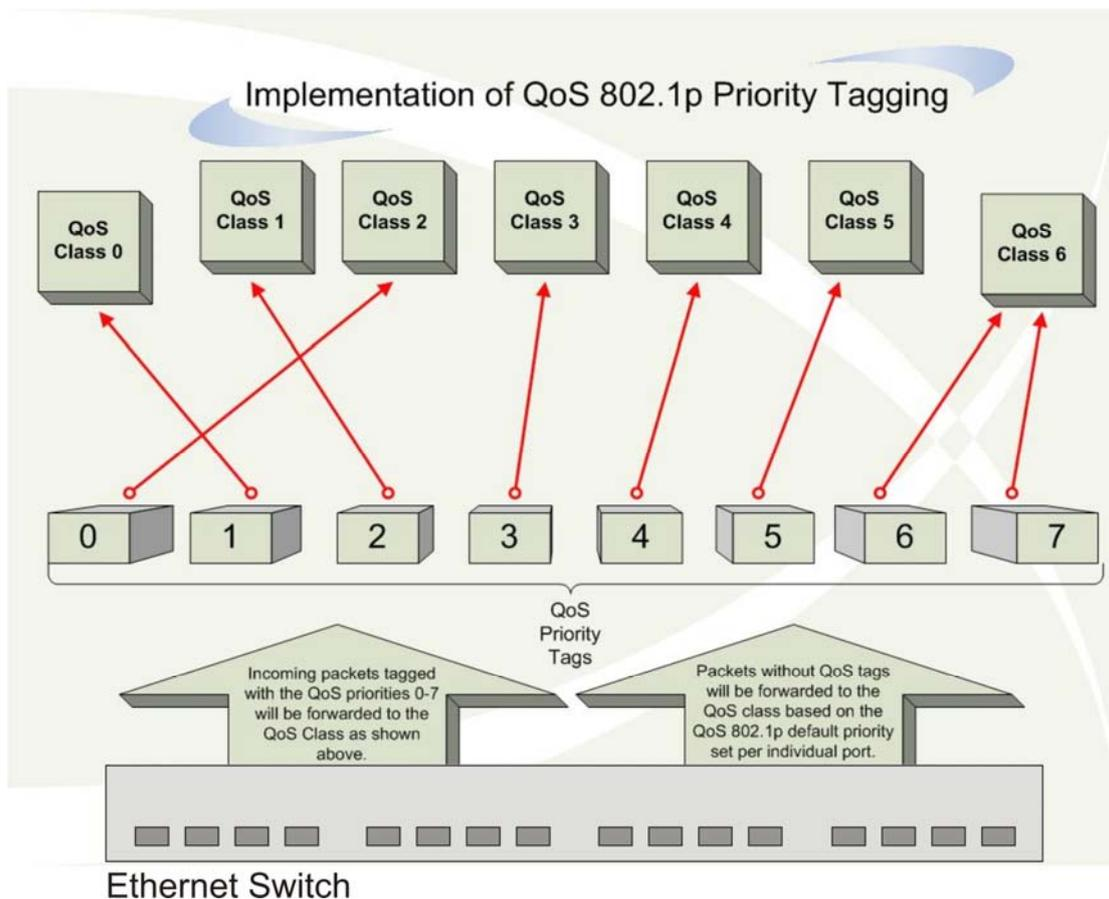
**Figure 5- 1. Mapping QoS on the Switch**
