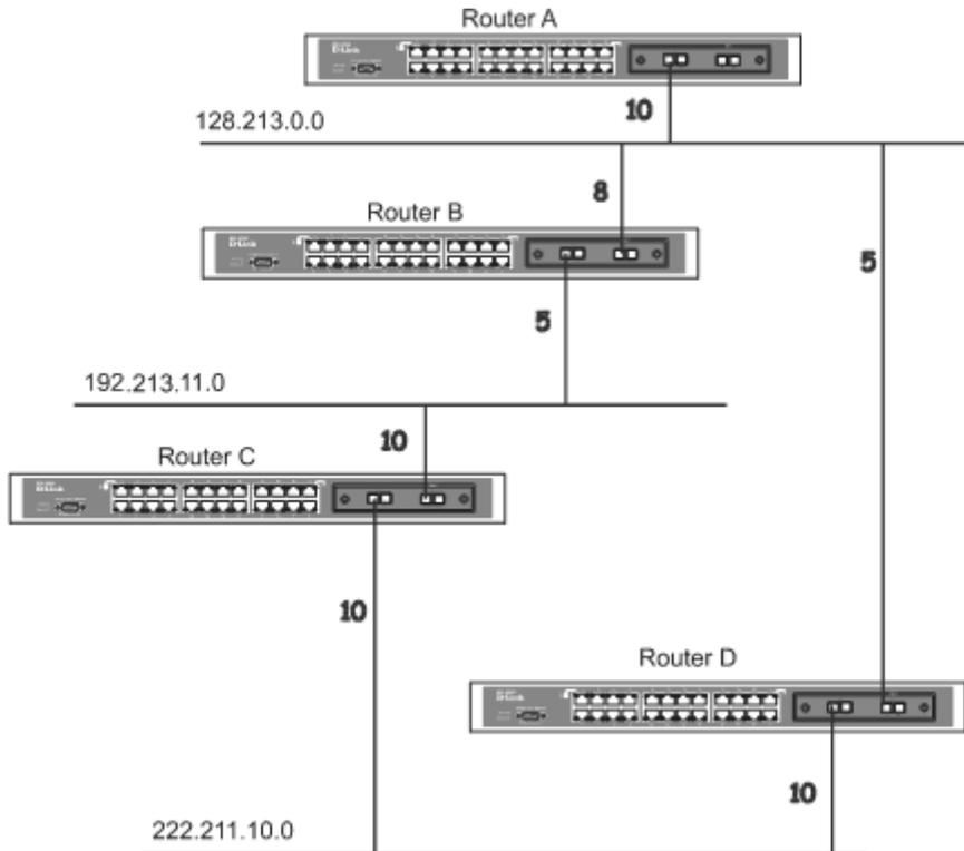
Figure 4- 36. Constructing a Shortest Path Tree
