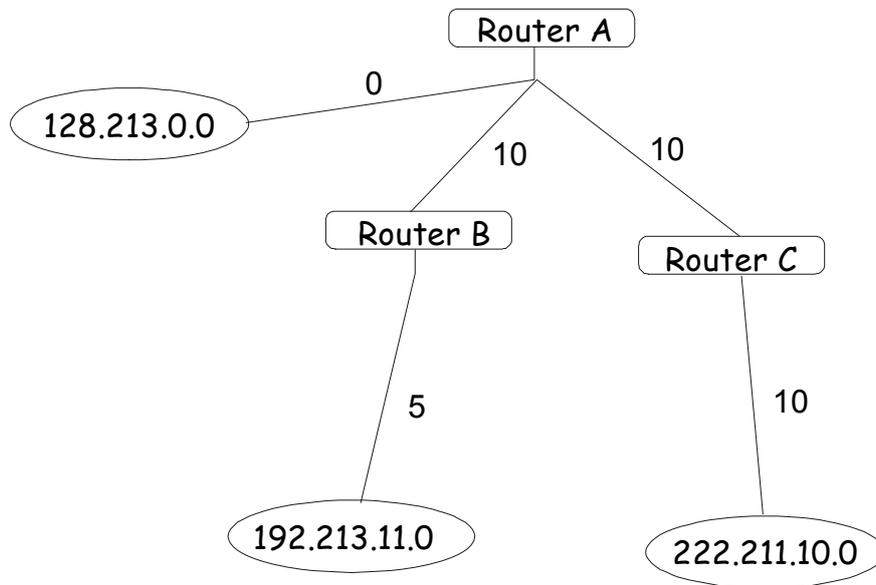
**Figure 4- 38. Constructing a Shortest Path Tree - Completed**
