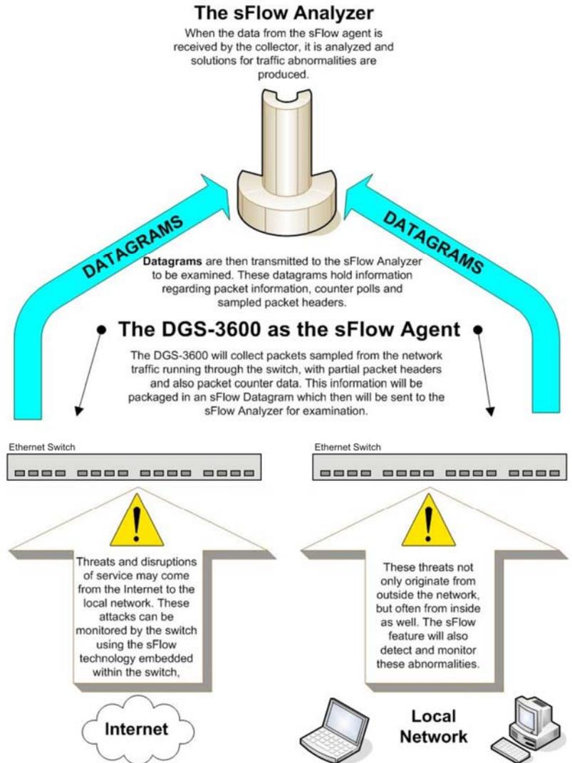
Figure 2- 81. sFlow Basic Setup
