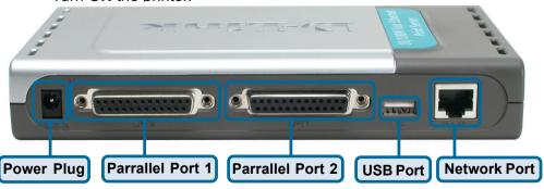
Then, plug one end of the power adapter into the DP-300U and the other end into your electric outlet.
