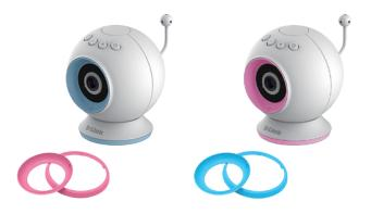
First choose the colour of the accent ring. To remove the accent ring simply turn counter clockwise to lift off. Then Place the new accent ring on, and rotate it clockwise until it clicks into place.
