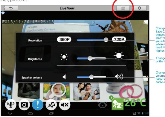
Change your EyeOn Baby Camera resolution between 360P and 720P. 360P resolution will give you a faster response, whereas the 720P resolution will give you a higher resolution image.
