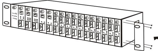
**Step 2:** Carefully position the chassis into the rack. Align the brackets to the side holes on the rack and use rack screws to secure the chassis with the rack.
