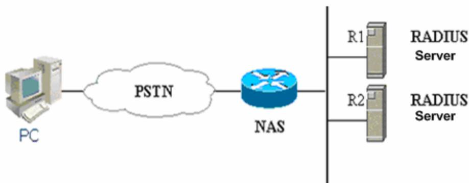
The figure above illustrates a typical AAA network configuration, including two security servers: R1 and R2 are both RADIUS servers.
