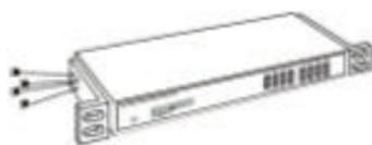
Figure 1. Combine the Switch with the provided screws.
