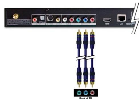
The **VIDEO OUT** button on the remote control toggles between the composite/S-Video output and the component video output. If component connectors are used but not selected, the screen will be tinted blue.
