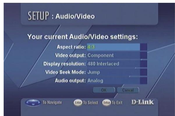
**Display Resolution:** If **HDMI** or **Component** is selected from **Video Output**, then the following five options will be made available: **480 Interlaced**, **480 Progressive**, **720 Progressive**, **1080 Interlaced**, and **Auto Detection**. If **Composite** is selected from **Video Output**, then the only option made available will be **480 Interlaced**.
