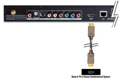
**Note:** *The first time you plug in this cable, you will need to press the **Video Out** button on the remote control several times until a video signal is received.*
