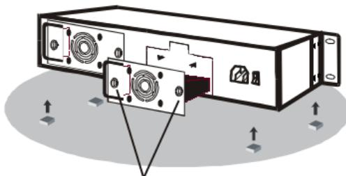
You can slide in and out the power supply from the bay, fasten or loose the hand screw clockwise or counter clockwise by using hand or screwdriver.
