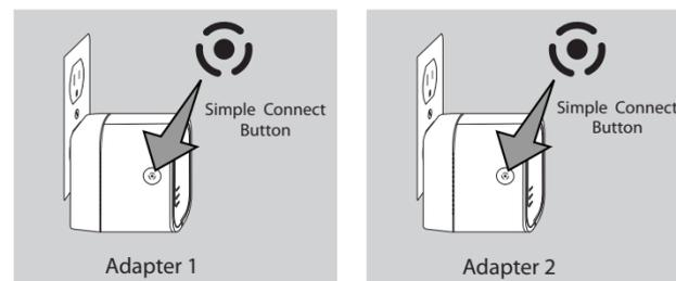
To secure your network, press the Simple Connect button for 2 seconds on one of the adapters. The Power LED will start to blink. Then, within 2 minutes, press the Simple Connect button on the other adapter for 2 seconds.
