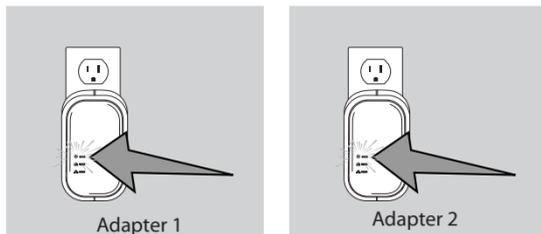
Plug one PowerLine AV Mini Adapter into an AC wall outlet. Verify that the Power LED is lit. If not, insert into another outlet. Now plug the other PowerLine AV Mini Adapter into an AC wall outlet. Verify that the Power LED is lit.
