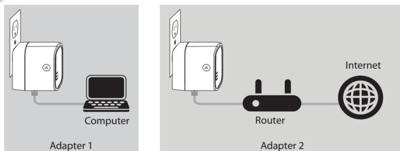
You may now attach Ethernet devices such as a router, computer, or game console via an Ethernet cable. With the Ethernet device powered on, verify that the Ethernet LED is lit on the adapters to indicate a good connection. Setup is complete.
