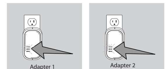
Once the Power LEDs stop blinking, verify that the PowerLine LED is lit on both adapters. This indicates that your adapters are properly connected to each other. If the LED is not lit, insert one or both adapters into different outlets and repeat step 2.
