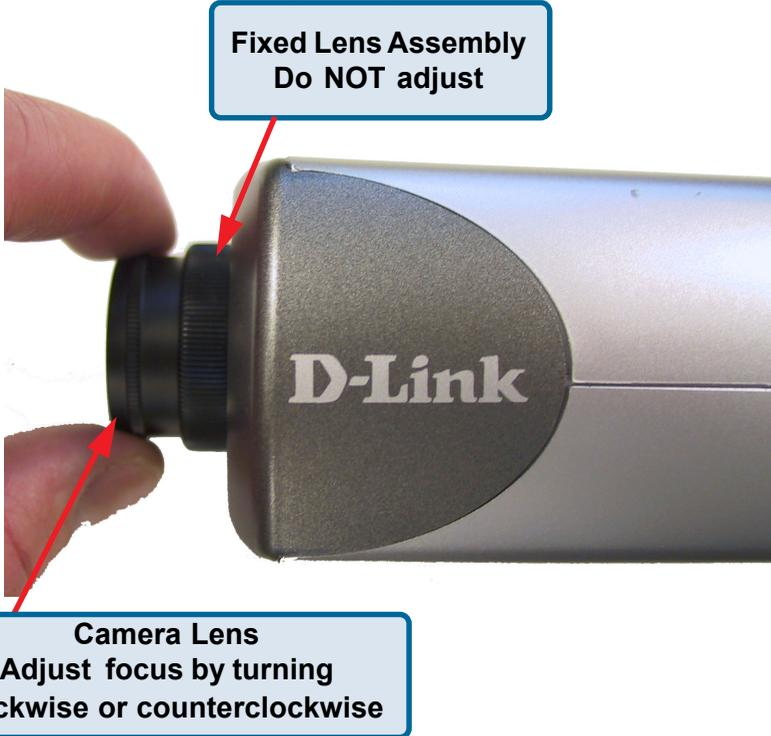
To adjust the focus of the lens you will need to turn the lens slowly either clockwise or counterclockwise until the desired image appears. **DO NOT** overturn the lens in either direction as it will be out of focus. Unless you want to substitute the lens **DO NOT** unscrew more than 1.0mm apart from the Fixed Lens Assembly.
