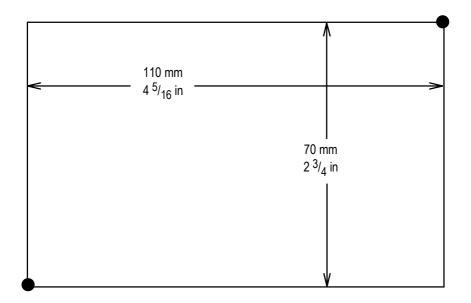
When setting the screws into the wall or partition, leave about 3 mm (1/8 in) between the head of each screw and the wall surface. Then place the DP-100 so that the mounting sockets on the bottom of its case fit over the two screws. Press the case gently toward the wall and slide the case at a  $45^{\circ}$  angle downward and leftward to engage the screwheads in the slots of the mounting sockets.
