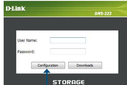
When logging into the DNS-323 for the first time, you will be asked to choose a drive configuration and format the drives. There are four options: **Standard**, **JBOD**, **RAID 0** and **RAID 1**. Standard configures each disk as a separate volume, while JBOD combines both disks into a single volume. See page 45 for more details on using the RAID configurations.
