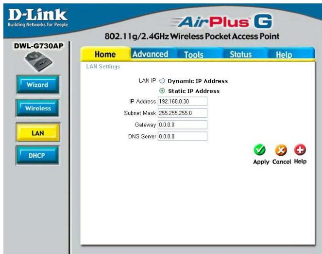
**Dynamic IP Address:** Select this option if you would like to have an IP Address automatically assigned to the DWL-G730AP by a DHCP server in your network.
