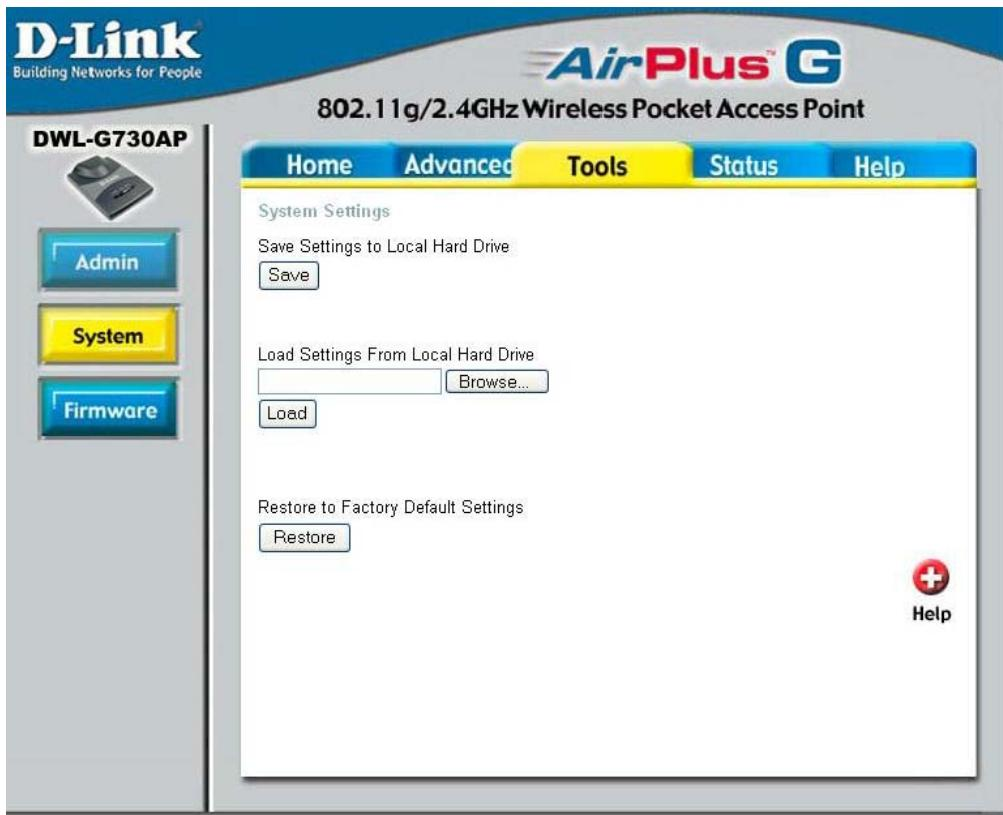
The current system settings can be saved as a file onto the local hard drive. To reload a system settings file, click on **Browse** to browse the local hard drive and locate the system file to be used.
