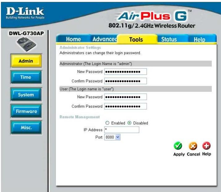
At this page, the DWL-G730AP administrator can change the system password. There are two accounts that can access the router's Web-management interface. They are **admin** and **user**. **Admin** has read/write access while **user** has read-only access. The **user** can only view the settings but cannot make any changes.
