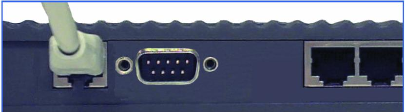
Using CAT5 UTP cable, connect each computer that is equipped with an Ethernet adapter to one of the **four Ethernet LAN** ports on the DI-704P.
