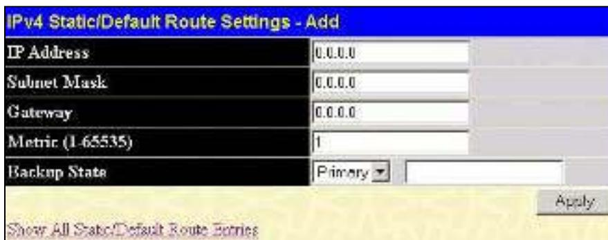
Figure 8- 10. IPv4 Static/Default Route Settings – Add window
