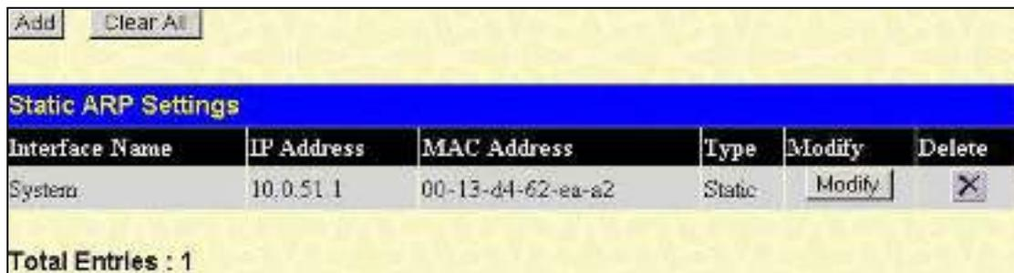
Figure 8- 13. Static ARP Settings window
