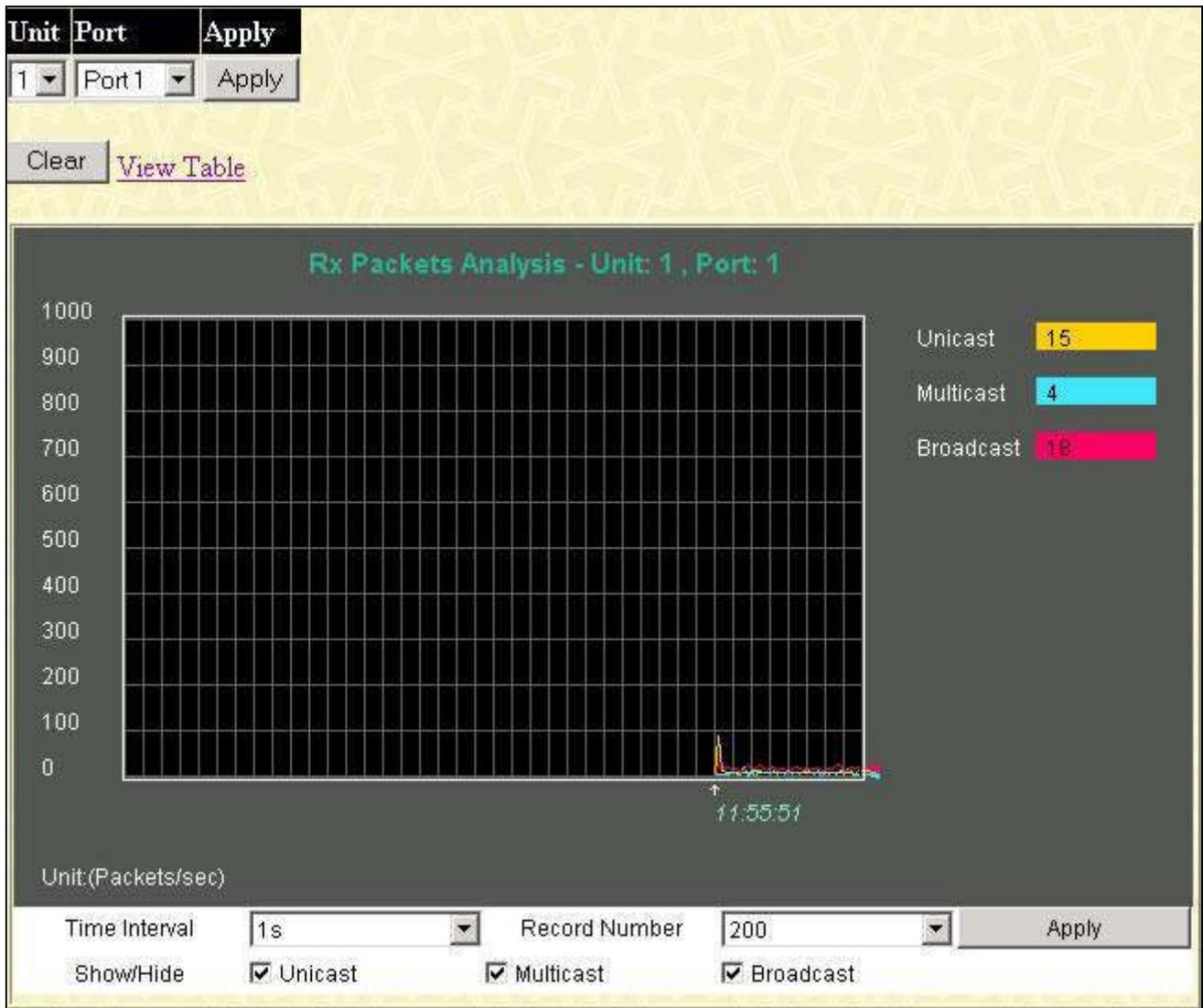
**Figure 12- 8. Rx Packets Analysis window (line graph for Unicast, Multicast, and Broadcast Packets)**
