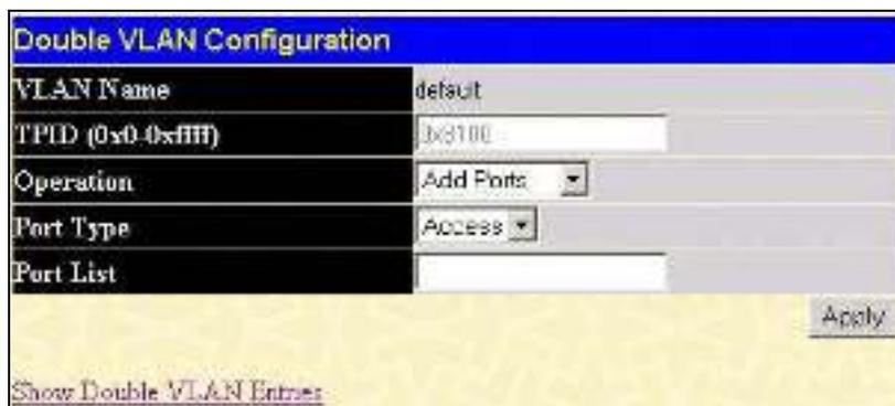
**Figure 7- 14. Double VLAN Configuration window**
