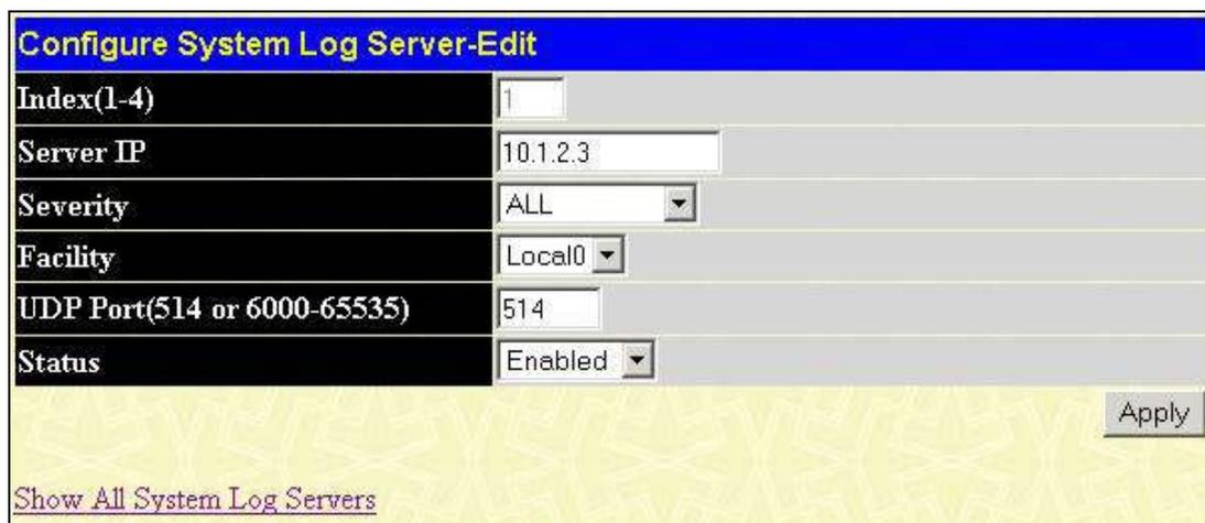
Figure 6- 15. Configure System Log Server– Edit window
