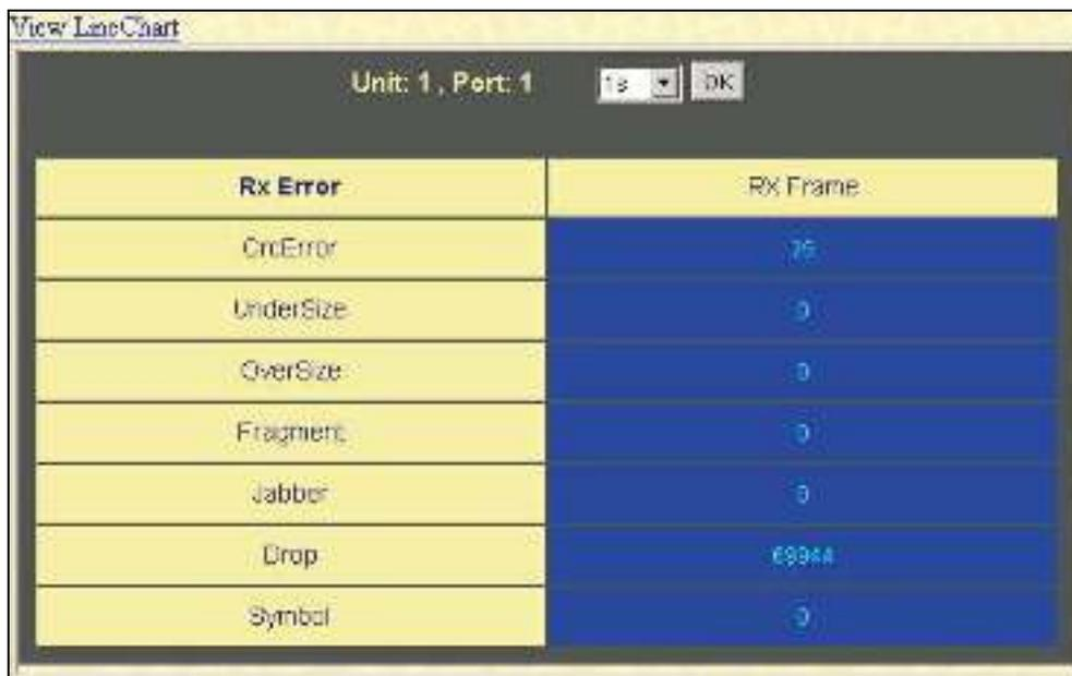
**Figure 12- 13. Rx Error Analysis window (table)**
