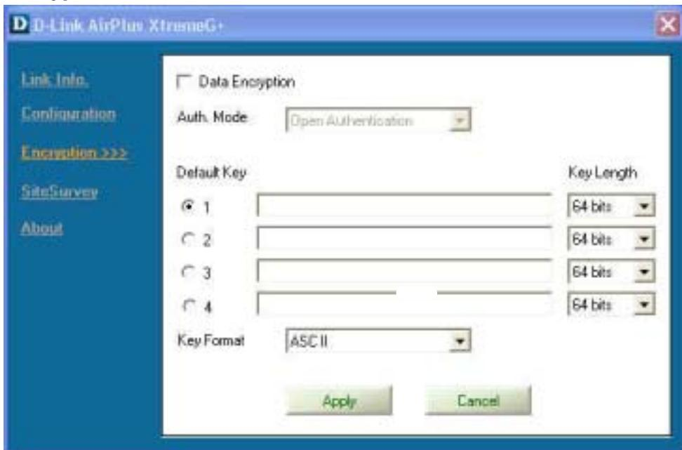
**Data Encryption** – enable Encryption by clicking on the box. Encryption is disabled as the default setting.
