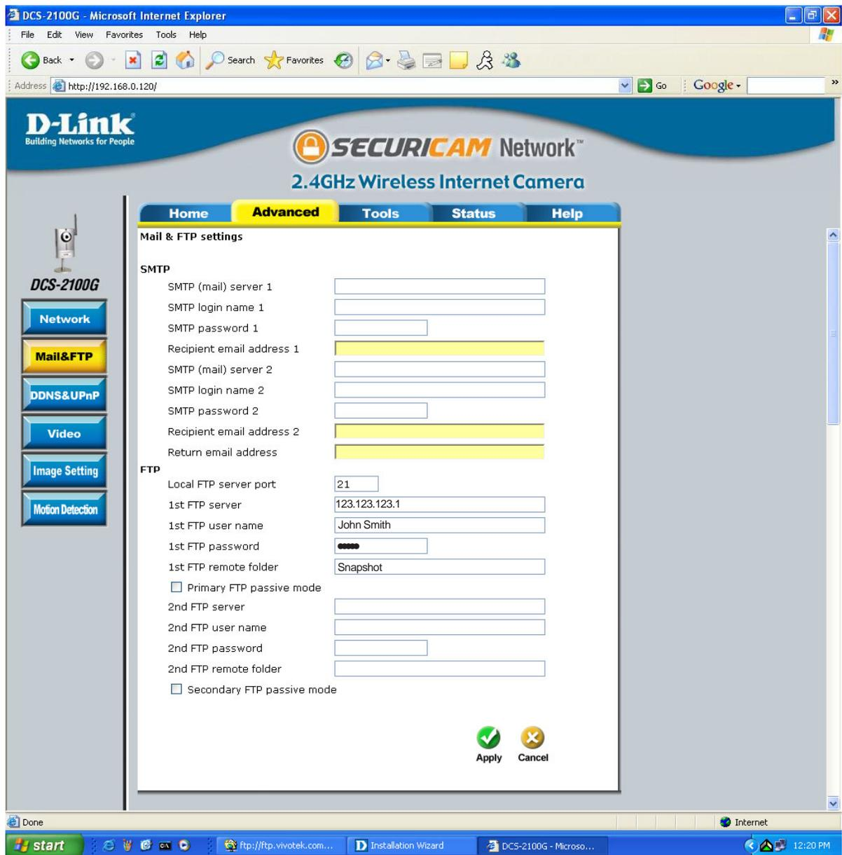
In this window, enter the settings for the FTP server you wish to record to. Optionally, you can enter settings for a secondary backup FTP server.
