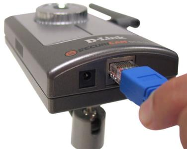
If you are connecting the **DCS-2100G** to a **802.11g wireless** Ethernet network, attach the one wireless antenna to the antenna connector on the side panel of the **DCS-2100G**.
