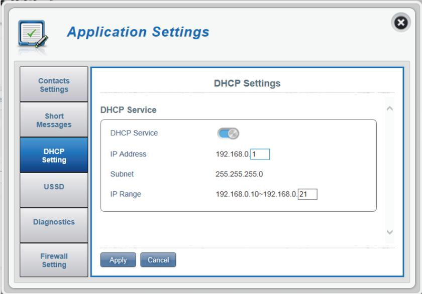
The screenshot shows the 'Application Settings' window with the 'DHCP Settings' tab selected. The 'DHCP Service' is enabled (toggle switch is on). The 'IP Address' is 192.168.0.1, the 'Subnet' is 255.255.255.0, and the 'IP Range' is 192.168.0.10~192.168.0.21. There are 'Apply' and 'Cancel' buttons at the bottom.
