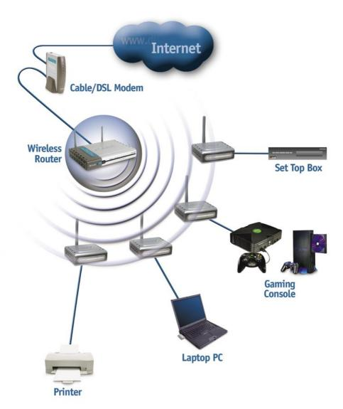
This example illustrates an **Infrastructure** setup. To connect the DWL-G810 to a wireless network with a wireless router or access point, please refer to the printed Quick Installation Guide included with the product. Web configuration is required to
