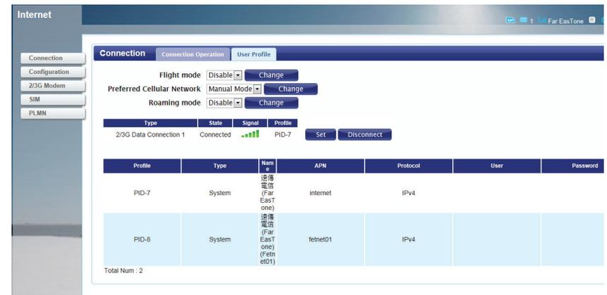
**Connection:** Shows the type and status of the current mobile connection. To change the connection profile, select a user profile from the table below and click **Set** to activate the profile. Click **Disconnect** to manually disconnect the current mobile data service.
